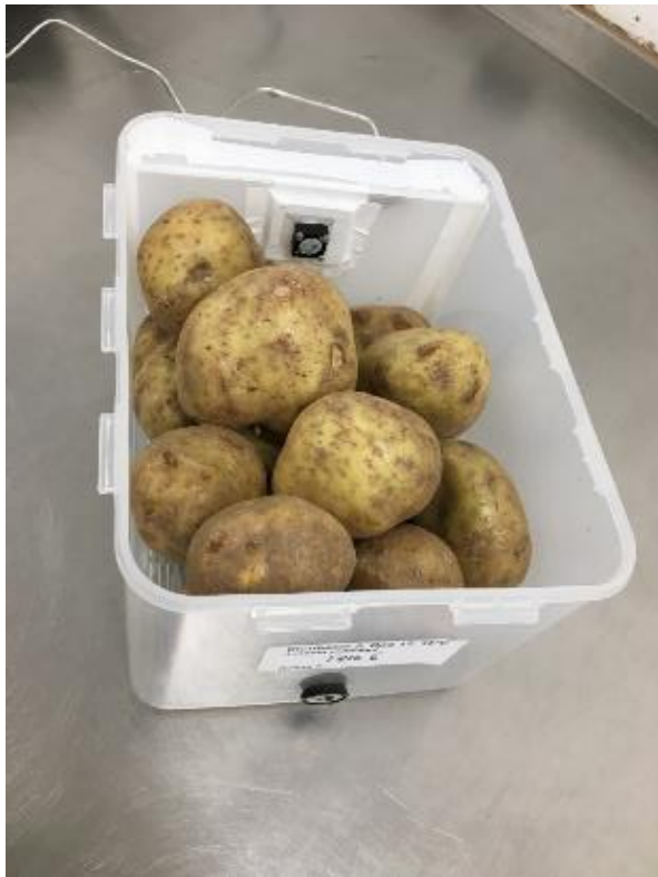
Figure 3. Individual positive ventilated plastic box. Air was pulled by internal fan from the plenum into the main chamber and recirculated through the potatoes (actual potato samples not shown) back via a box-wide opening at the bottom of the plenum. Limited external air exchange (estimated 8 chamber air changes per day) was enabled via an external vent into the plenum and outlet via vent at the front of the box. Box lid not shown.
